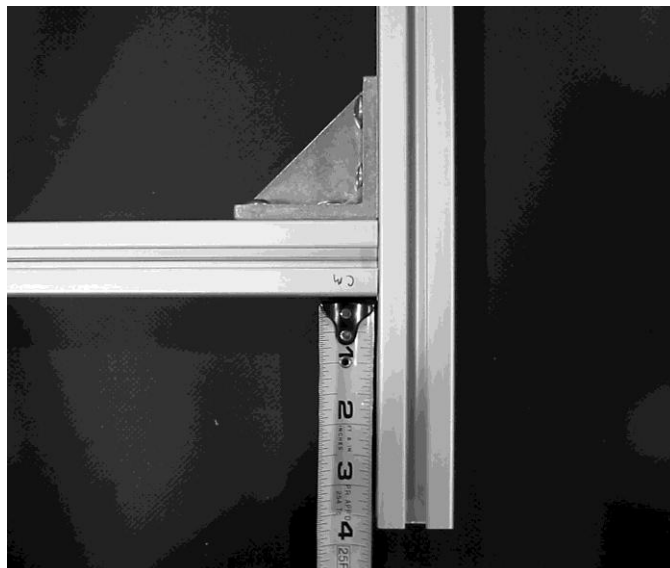
Photo #6 (Left Vertical to Bottom Cross Member)
